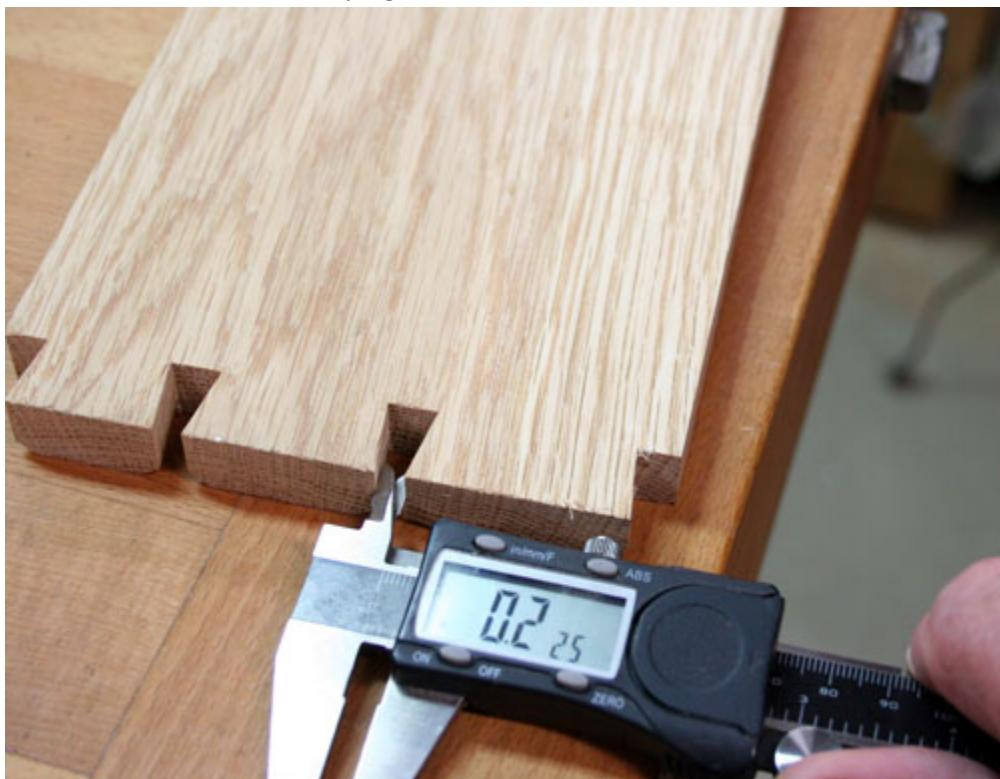
36. It is lengthy to explain the mechanics, but the offset calculation is width of our dovetail bit minus width of the top opening in the tail board divided by 2 then the result is added back to the width of the top opening. In this case all offsets are to be .300"
