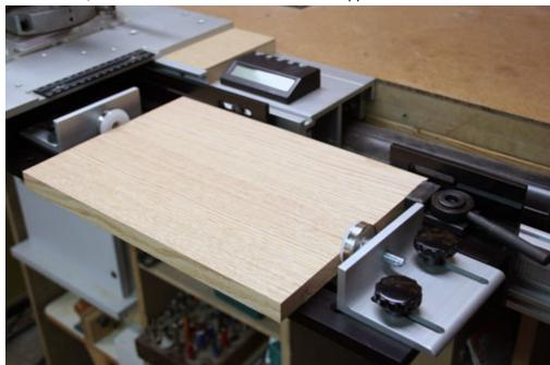
5. We'll make a stopped sliding dovetail like those most often used in the sides of bookcases. Mark a line on the board where the dovetail socket (slot) will stop. Mark a corresponding line on both sides of the Router Boss base plate. We'll use this line to position the angle guides.
