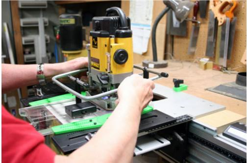
14.15. We have now completed the dovetail slot for the tapered sliding dovetail. This is actually the easier part and can be repeated if you have other slots to cut. Next we'll measure the taper and setup for the tenon cut.
