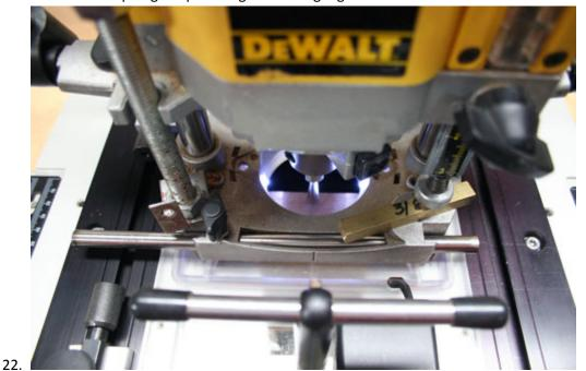
23. Use the built-in laser cross-hair to position bit at approximately the center of the tenon board. Slide the 2 precision stops against the router stop bar and lock both in place. Also lock Router Boss's router plate with the star knob.
