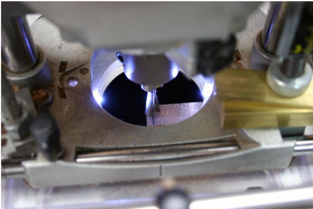
28. Complete all tail board cuts at the logged cut locations. Cut slowly so as not to break the dovetail bit. I do a climb cut when making the half-pin cuts on each side by starting the left half-pin from the front of the board and the right half-pin from the rear of the board.
