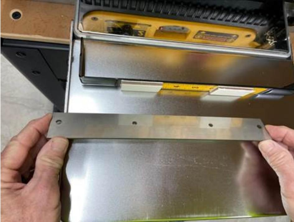
Gently **slide** the DRO backplate onto the six-inch scale and note the **two parts' needed alignment**, as shown in the photo below. The lower edge (right-hand side in the picture) of the backplate should be aligned with the bottom edge of the DeWalt yellow six-inch scale as shown below:
