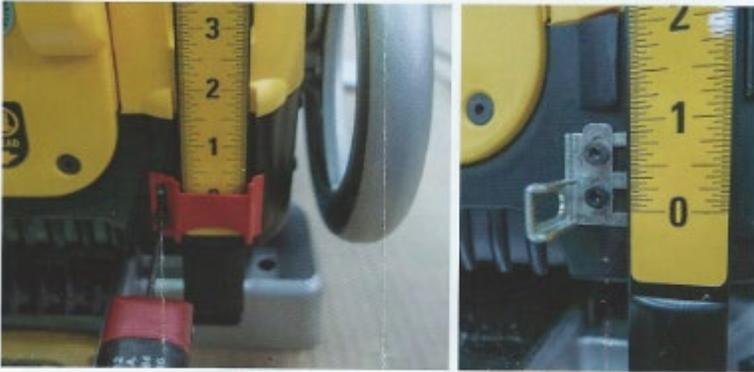
Step 2: Install side lever on DRO then attach the assembled unit on the DeWalt yellow rule, as shown below using VHB tape and spacers. The sheet metal back should align with left edge of the yellow rule. The bottom cap screw should be about 1/4 inch below the 0 mark on the rule.
