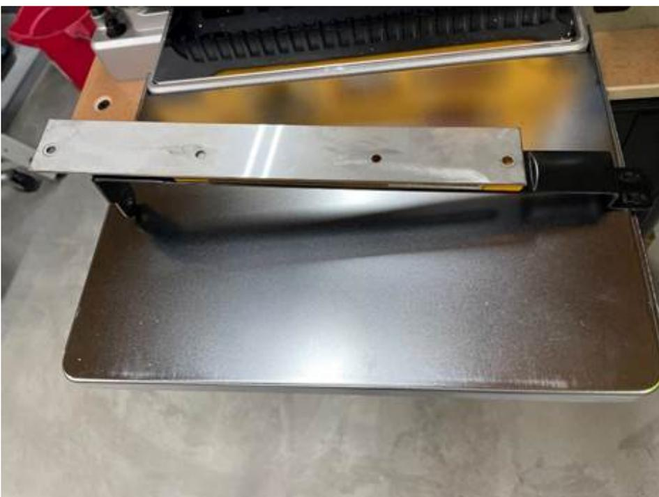
Now you are ready to reassemble the DRO scale to the backplate. This part is straight forward with one exception. The lower screw and hex nut are not easily accessible when attaching the DRO onto the backplate. The assembly is best done with an 8 mm combination wrench or needle-nose pliers to hold the hex nut before tightening. Here is a photo:
