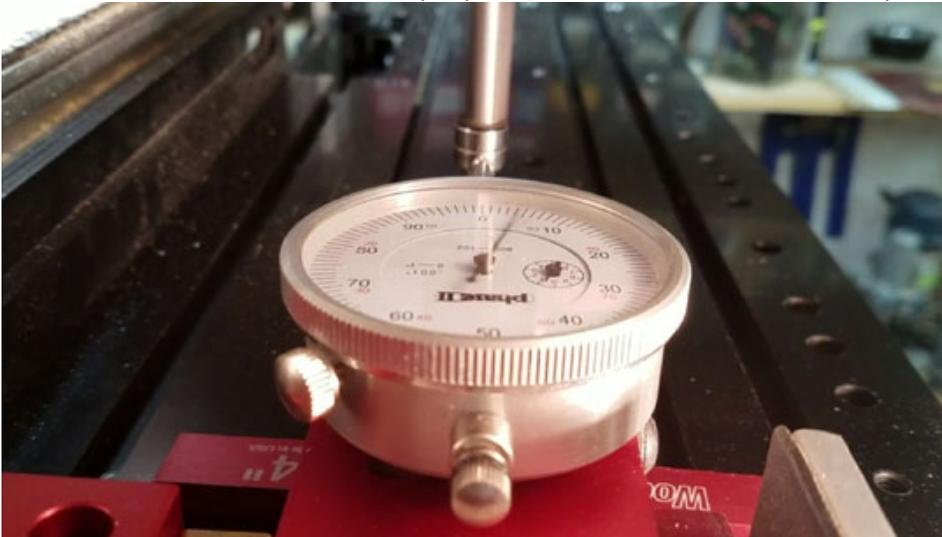
The bottom line was I would say the deflection was .006 +/- .003 for both extenders -- running at speed 2 did not improve the run out -- the only difference between the two is that manually spinning the CMT shows +/- .001 and the Chipsfly shows +/- .002 -- as the router slows from speed to stopped the CMT seemed smoother than the Chipsfly -- for whatever reason --
