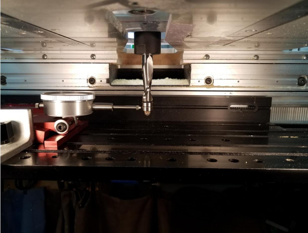
I used a Freud 75-508 1 1/4" flush trim up-cut spiral bit with an end bearing -- just the bit chucked, no extender. Manually spinning it yielded +/- .001 deflection -- at speed 5, I read .003 +/- .003 -- the needle bounced from 0.0 to .005 or so -- reducing the speed to 1 did not change the amount of deflection, but the movement of the needle was less active --
