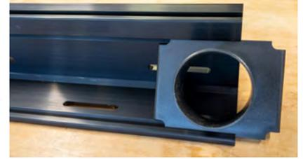
Place a button-head 1/4-20 bolt through each countersunk front hole in one fence face and the front slots in the aluminum fence. On the back side of the fence, screw two of the round knobs onto these bolts. Repeat for the other fence face.
