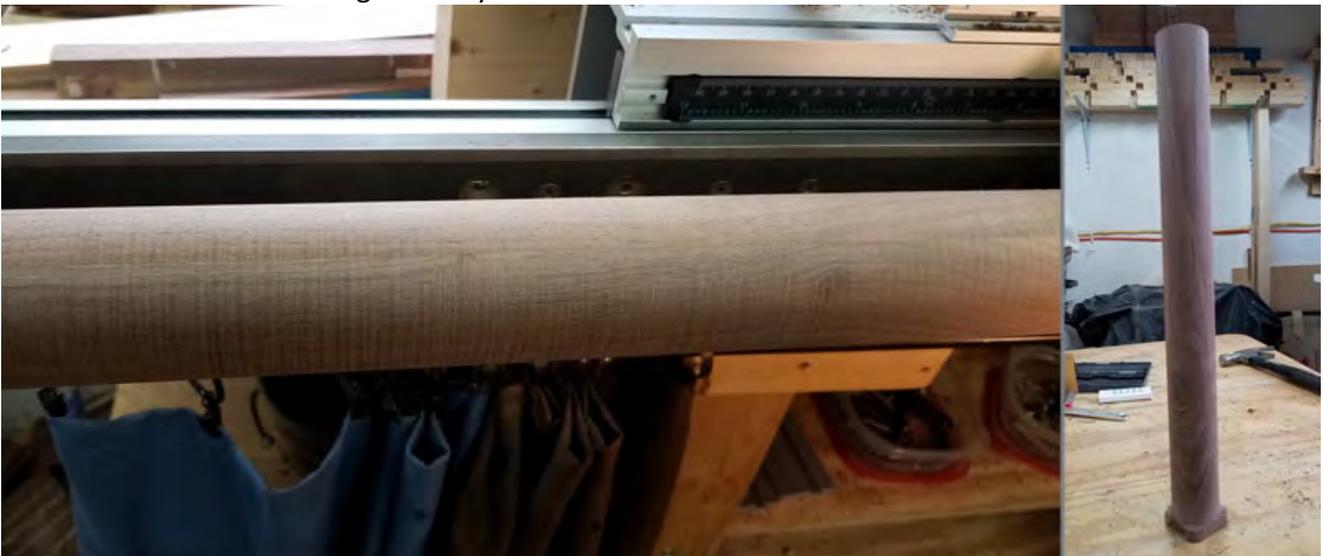
A few thoughts on the cutting process -- I rotate the piece away from me -- clockwise looking from the head stock -- I think that is the 'normal' router cut -- rotating the wood into the rotation of the bit
