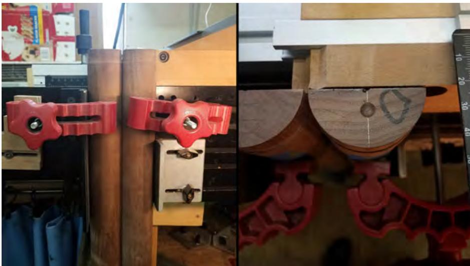
cut on each of the 22" pieces -- the columns were turned to 2" (+/- 1/128) so they would match -- the half cuts were done to maintain the 1" radius -- side panels are 2.5" wide
