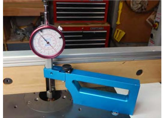
To set cutting depth place fence in approximately the desired position. With SNAP-CHECK PRO on its side, place the base against the fence and the anvil gently on the cutter. Rotate the bit to find top dead center. Adjust fence position to achieve the exact desired cutting depth.
