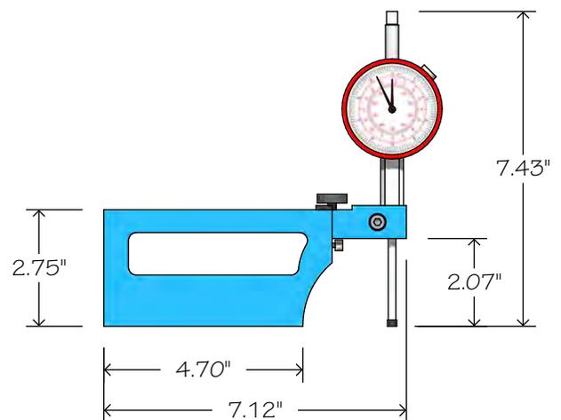
Flat, Extended Flat & Ball anvils included. Replace flat anvil with ball anvil when measuring moving objects. Use extended flat anvil for depth measurements up to 1/4".
